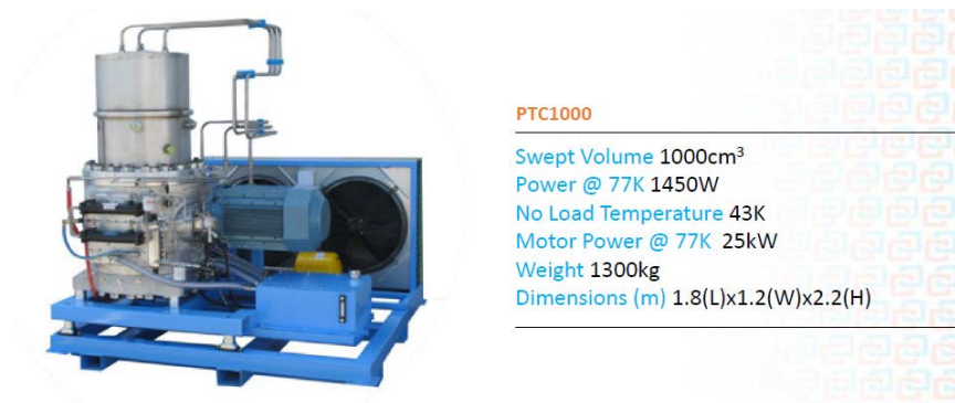
Figure 4: Example of pulse tube cryocooler delivering a cooling power of 1450 W@77K
