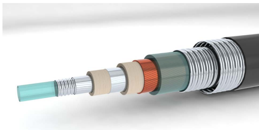
Figure 14. A 1 GW power link comprising one HTS cable with 2 symmetric poles. Here a cooling fluid return line is needed but not represented. Pole 1 = 10 kA@+50 kV and Pole 2 = -10 kA@-50 kV)
