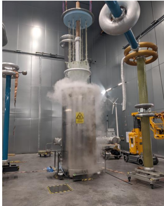
Figure 42: Limitation test on superconductive tape sample.
