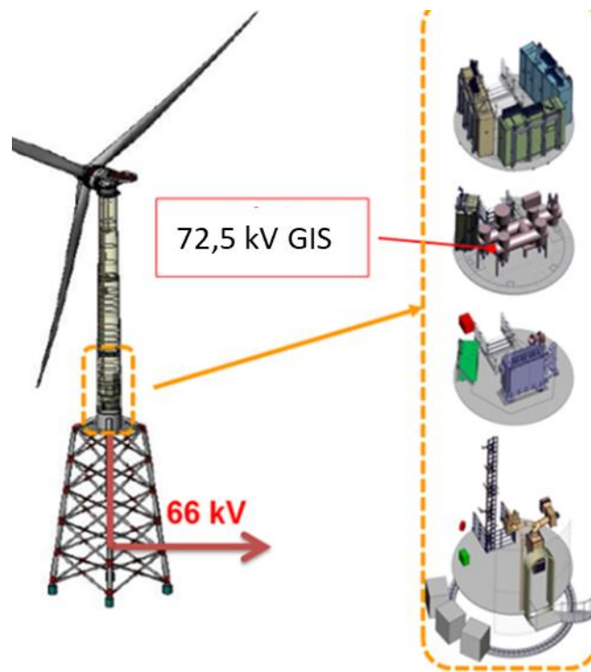
Figure 21 : A possible wind turbine electrical arrangement. The converter and transformer are typically located inside the nacelle, next to the generator, whereas the high voltage switchgear may be placed inside the mast.
