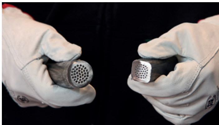
MgB2 superconductors during one of the manufacturing stages
